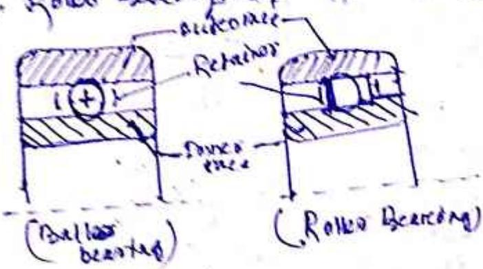
→ The Ball & Roller bearing consists of an inner race which is mounted on the shaft or journal & the outer race, which is carried by the housing or casing.
