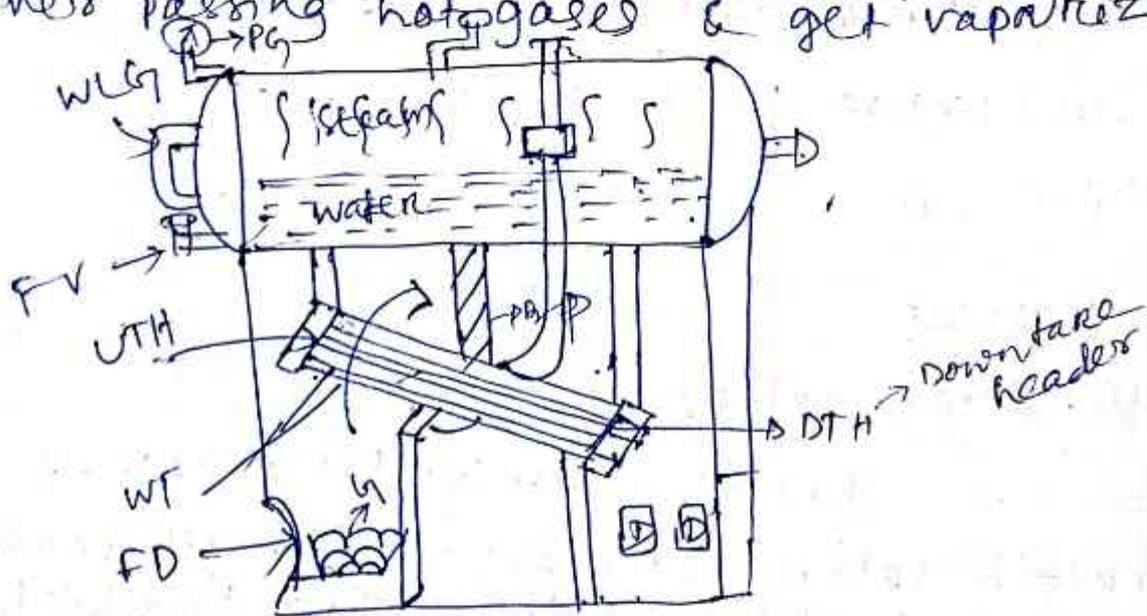
When we start moving from down take Header start to move uptake header & then the steam is collected at the steam stage uptake header.
