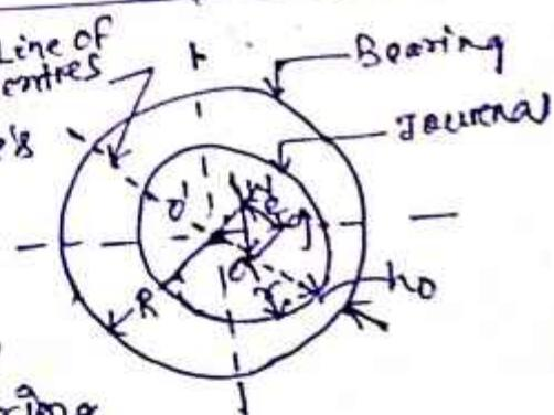
1. Diametral clearance :- It is the difference bet<sup>n</sup> the dia. of the bearing & the journal.
