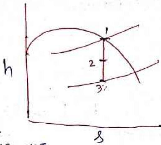
$$h_1 = h_g | 11 \text{ bar} = 2780 \frac{\text{kJ}}{\text{kg}}$$
