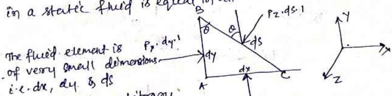
The fluid element is of very small dimensions i.e.  $dx$ ,  $dy$  &  $ds$ . Consider an arbitrary fluid element in a fluid mass at rest.
