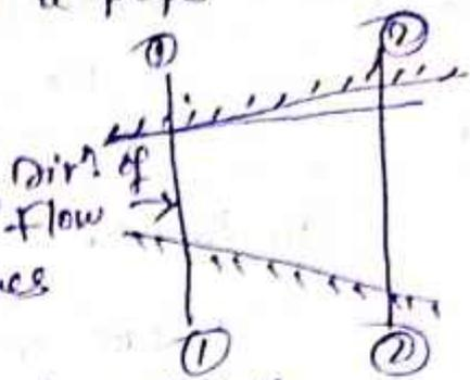
Then Rate of flow at section 1-1 =  $\rho_1 A_1 v_1$
