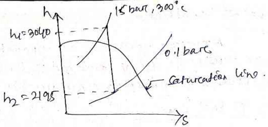
$$(\Delta h)_{\text{isentropic}} = h_1 - h_2 = 3040 - 2195 = 845 \frac{\text{kJ}}{\text{kg}}$$
