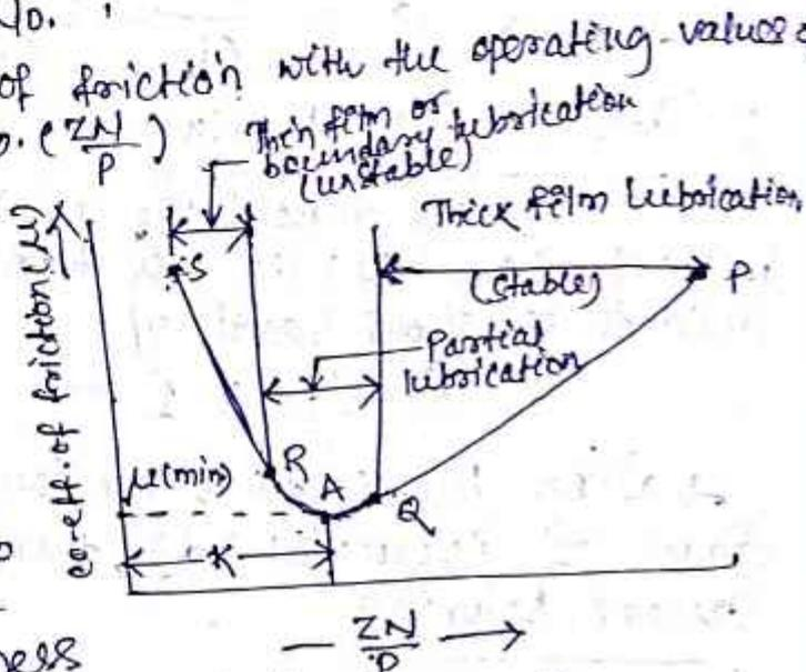
→ This will result in high friction, wear & heating
