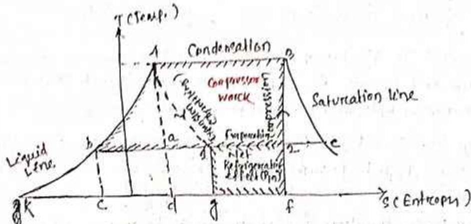
It then undergoes throttling expansion while passing through the expansion valve, and it again reduces to  $T_2$ , it is represented by the line 4-1 shown broken; due to this expansion the liquid partially evaporates, as its dryness fraction is represented by the ratio  $\frac{b_1}{b_2}$ .
