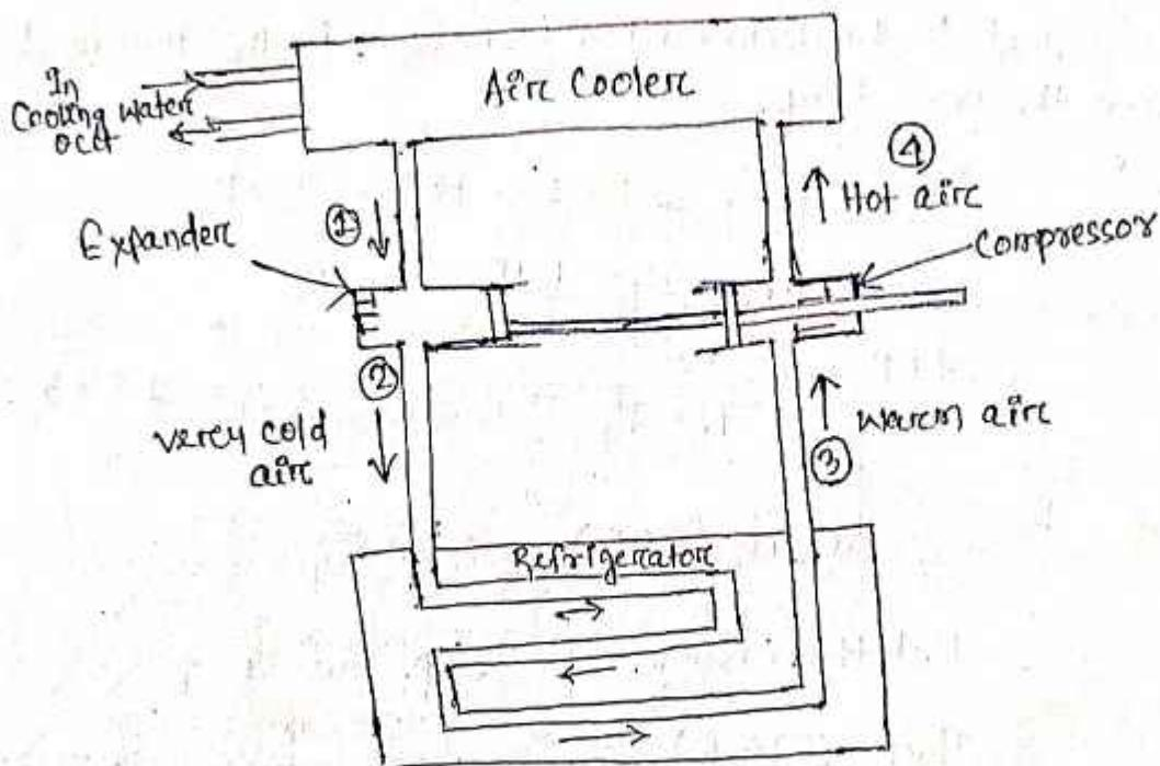
Schematic diagram of an air-refrigeration System working on the reversed Brayton (or Bell-Coleman or Joule) cycle.
